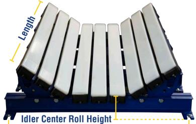
Impact Bed to be installed minimum of 1/2" lower than idlers. Belt should only make contact with impact bed under load.
